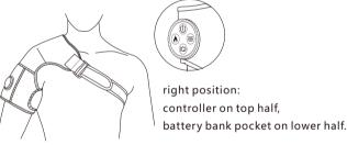
(3) press power key 2 sec. allfunction working, green light open (4) press heating key:low/middle/high/off (light color:green/blue/red) (5) press air pressure key: I mode/Imode/off (light color:green/blue/red) (6) press viberation: weak/pulse/steady/off (light color:green/blue/red)
